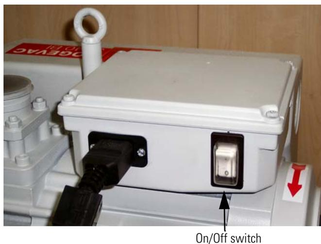
**Figure 1-17.** Forepump with On/Off switch
