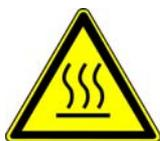
**Warning Burn Hazard.** Allow heated components to cool before you service them (the ion transfer capillary at about 300 °C, for example). ▲
