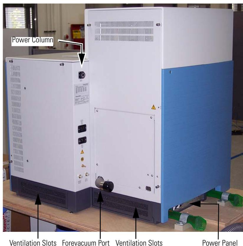
**Figure 1-4.** Rear side view of the instrument
