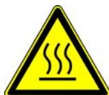
**Warning Burn Hazard.** If you abort a system bakeout, parts of the instrument can be hot. Allow the instrument to cool for at least three hours before you start operating it again. ▲
