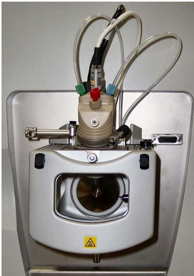
**Figure 1-7.** Ion Max ion source with ESI probe attached
