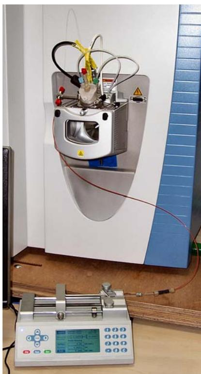
**Figure 1-14.** Exactive with Chemyx Fusion 100 syringe pump
