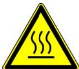
**Warning Risk of burn by touching.** Pump in function is hot and some surfaces could reach a temperature higher than 80 °C (176 °F). Take note of the warning labels on the pump. ▲
